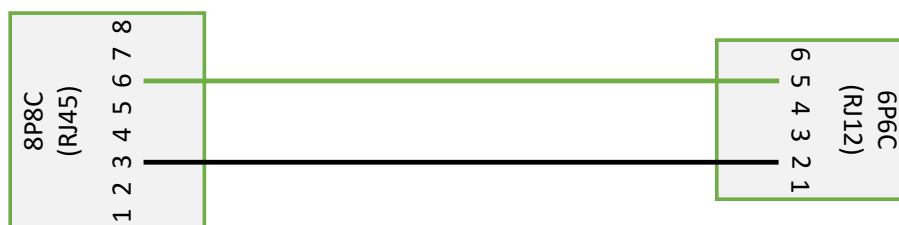
Fig. 31. Cable for 12 V power feed from X-BUS connector 3
